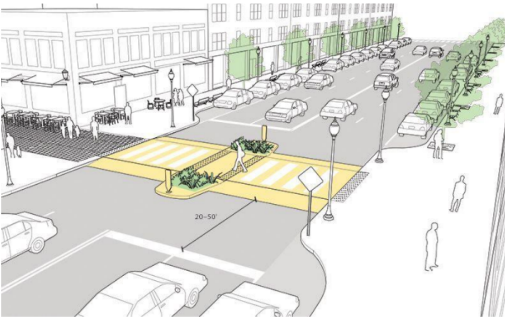
Fig 3.9 A typical intersections with essential elements
