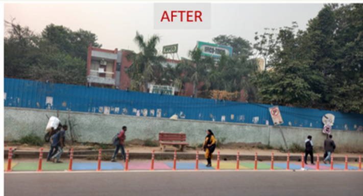
Painted zebra crossings & pedestrian pathways gave a designated space for pedestrians to cross roads & walk as well as a reference point for vehicles to stop before the signal.
