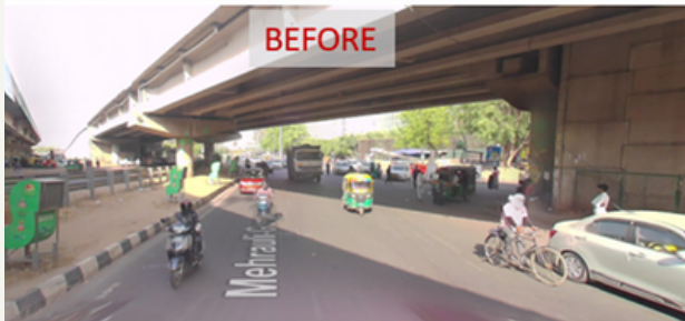
There was no traffic signal and pedestrian at-grade crossing at the junction, which was leading to haphazard pedestrian movement and high-speed traffic movement, leading to multiple conflict points.
